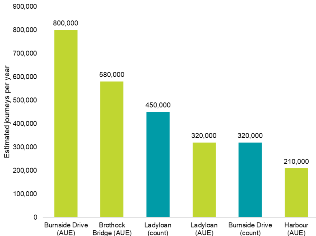
Figure 6: 365-day counts and annual usage estimates for active travel, at six locations in or around the project area
