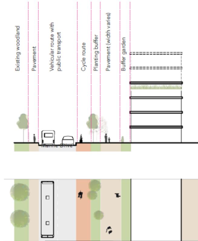
Fig. 5.23: Illustrative section and plan for Marine Drive / West Shore Road
