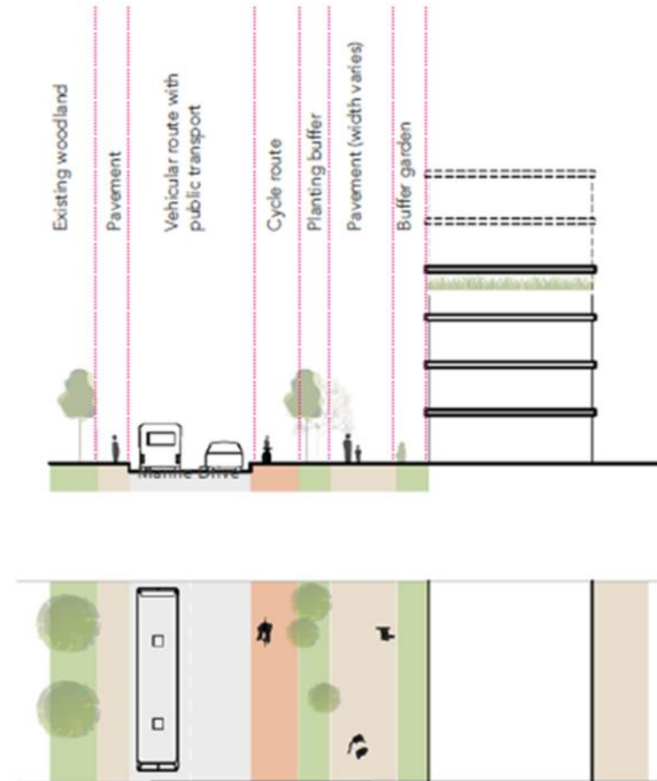
Fig. 5.23: Illustrative section and plan for Marine Drive / West Shore Road
