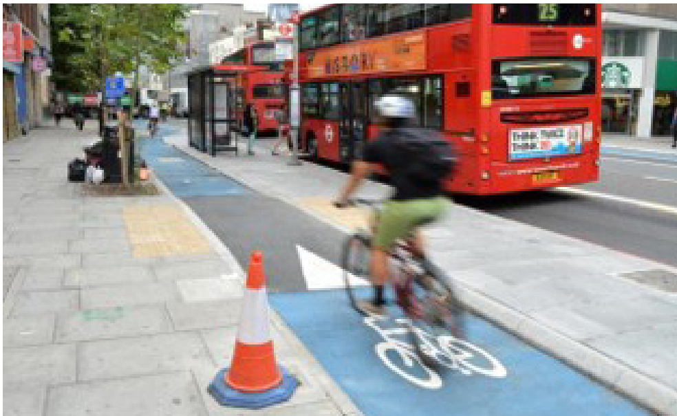
Figure 37. Crossing of one-way cycle track to access bus stop
